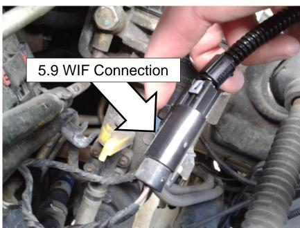
11. Turn the key on and wait for pump to prime the fuel filter before starting engine. Check for leaks from the sensor.
