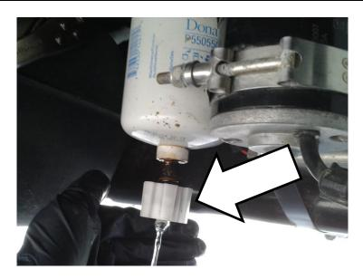
Replace the threaded adapter in the filter head with the new one included in the kit.
