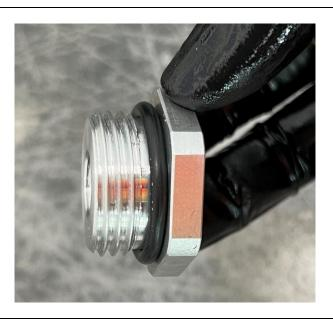
Check that the new WIF sensor O-ring is present, and then thread the sensor into the filter to WIF adapter.
