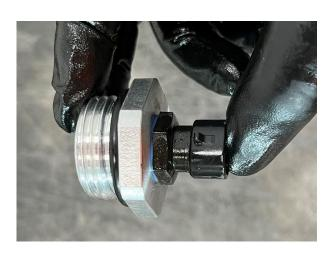
6. Install the WIF filter adapter and sensor into the water separator.
