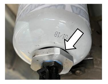
7. Connect BD wiring harness to the sensor and route the wire towards the engine bay.
